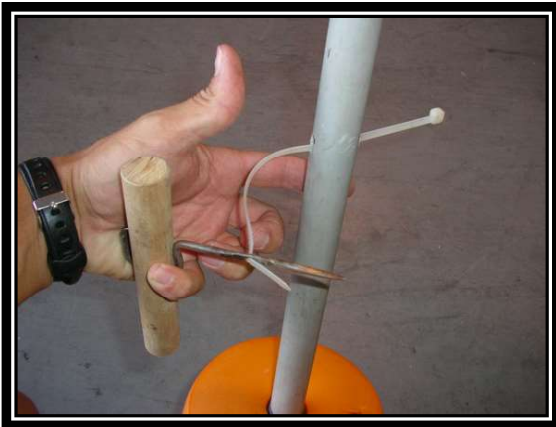
Fig 3. Tie pulled through line and pipe
