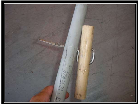
Fig 2. Awl through hole in pipe and line
