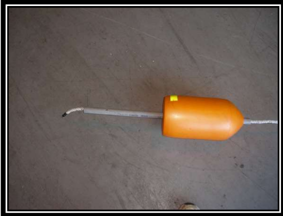
Fig 1. 14" buoy with PVC pipe dowel
