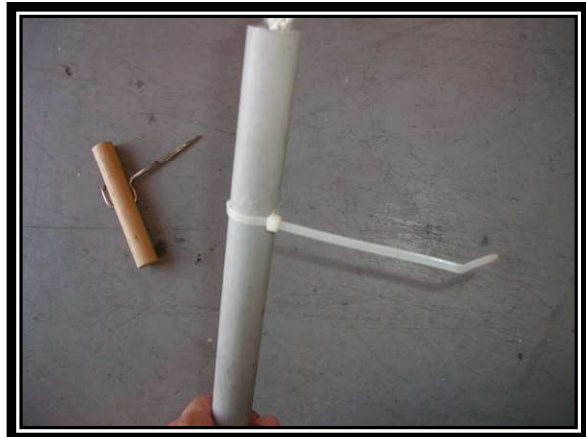
Fig 4. Remove awl and lock down tie
