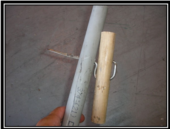
Fig 2. Awl through hole in pipe and line
