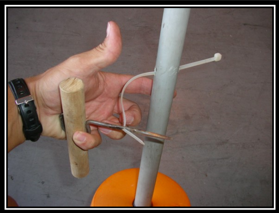
Fig 3. Tie pulled through line and pipe
